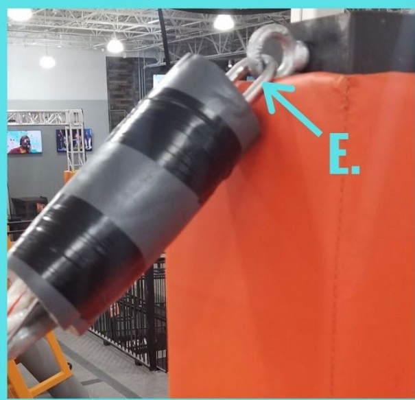
A. Fidget Ladder B. Pit (Air Bag Pictured) C. Anchor Posts D. Perimeter Padding E. Connection Hardware (Ladder to Post)
